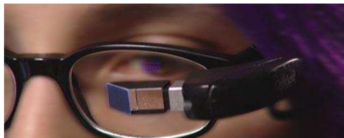
Figure 1. A wearable user's head-up display mounted on eyeglasses.
