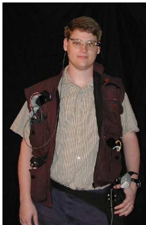
Figure 6. The Capture Vest and wearable computer worn by a user. The vest contains the hardware needed to capture the video from the user's perspective.
