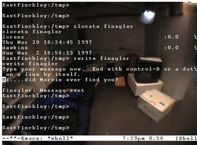
Figure 2. The user’s mind merges the images seen by the unoccluded eye and the eye with the opaque display. The resulting perception seemingly overlays the virtual on to the physical environment.
