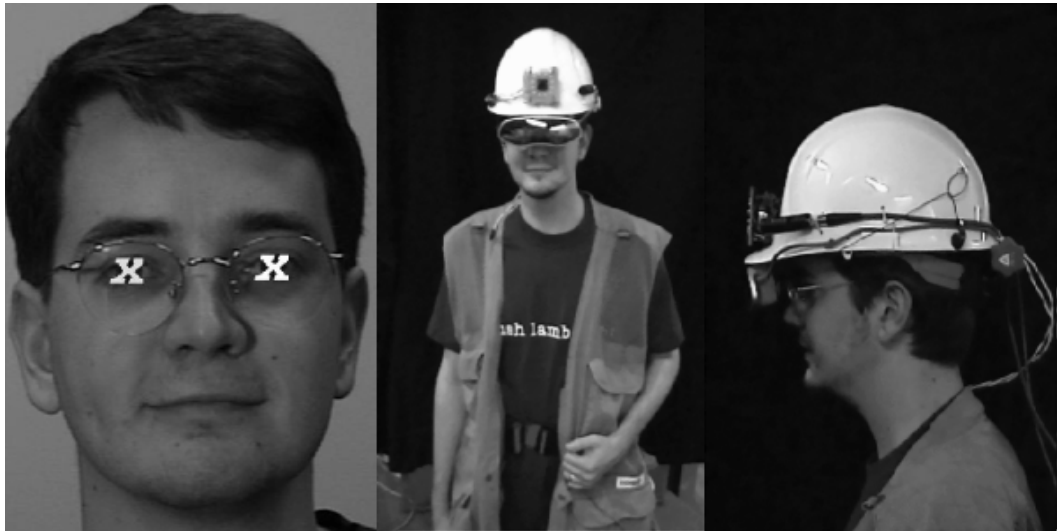
Figure 2: Marks for user alignment and face capture apparatus
