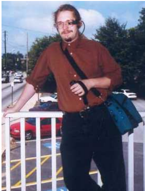
Fig. 1. Wearable computer user with MicroOptical SV-3 640x480 color display, 800MHz CharmIT Pro, and Twiddler 2 one-handed chording keyboard.
