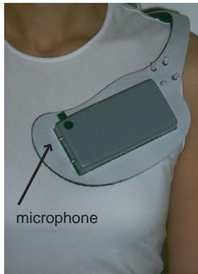
Figure 2-18: A “sociometer,” a portable audio/accelerometer/IR tag recorder developed by Tanzeem Choudhury, with the housing designed by Brian Clarkson. The microphone is about 6-7 inches away from the speaker’s mouth.
